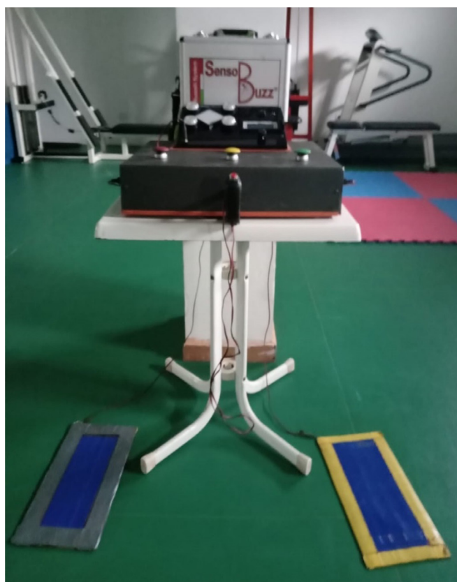
Figure 1. The figure shows the SensoBuzz console used to evaluate simple and complex reaction times.
