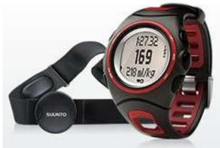
Figure 2. Sophisticated heart rate monitor capable of recording R-R intervals and the variations in such intervals over time.
